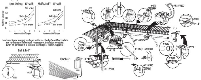
$\label{thm:components} Components \ provide \ for \ Closet \ Maid \ shelving \ installation \ to \ drywall \ without \ requiring \ mounting \ to \ wall \ studs.$
